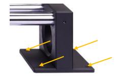
Adjust both side support with the 4 grub screws. The reel columns has to be parallel and levelled to the ground. For that use a spirit level. After that the sliding platforms have to be moved smoothly. (Screws are included)
