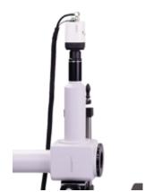
Insert the tube with the attached video camera, power- and BNC video-cable.
