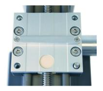
The four corner holes are for the screws to hold the measuring head. The centre block fits into the adaptor plate of the measuring head, in order to centre it on the spindle table.
