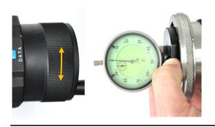
Turn the hand wheel of the digital micrometre un pointer of the test gauge matches "0"
