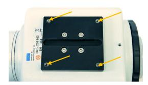
The adaptor plate on the bottom of the measuring head, in order to centre it on the spindle table. Move the spindle table as high as possible and put the measuring head on to it. It is **very important** to secure it with the four Allen screws (M5).
